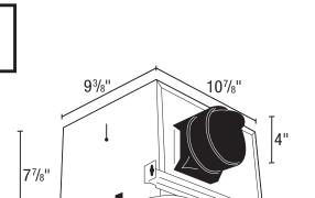
Acceptable for use over tub or shower when installed in a GFCl protected branch circuit.
