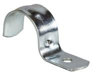
Rigid One Hole Straps are used to fasten Rigid or IMC conduit to wood, masonry, and other working surfaces. They are manufactured from carbon steel and feature an inverted rib on the backside for increased rigidity. They are zinc plated for increased corrosion resistance.
