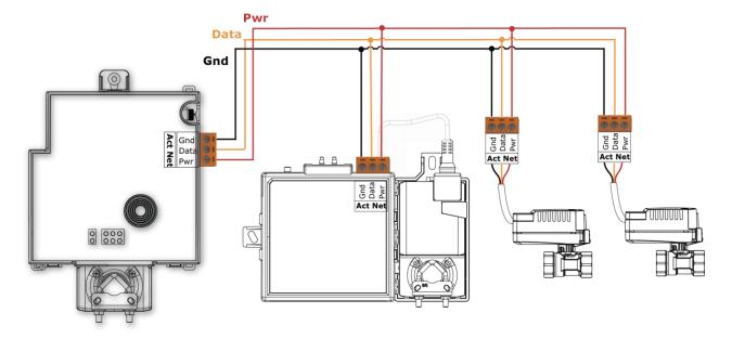
The TV-VVTBP-E2 supports Act Net communication to the Act Net devices on a bus with a maximum length of 300 feet (91.44 meters). The bus should be wired with copper conductors of an appropriate size (18 AWG or larger) to compensate for voltage drop and ensure that bus voltage does not drop below 19.2 Vac or 21.6 Vdc.
