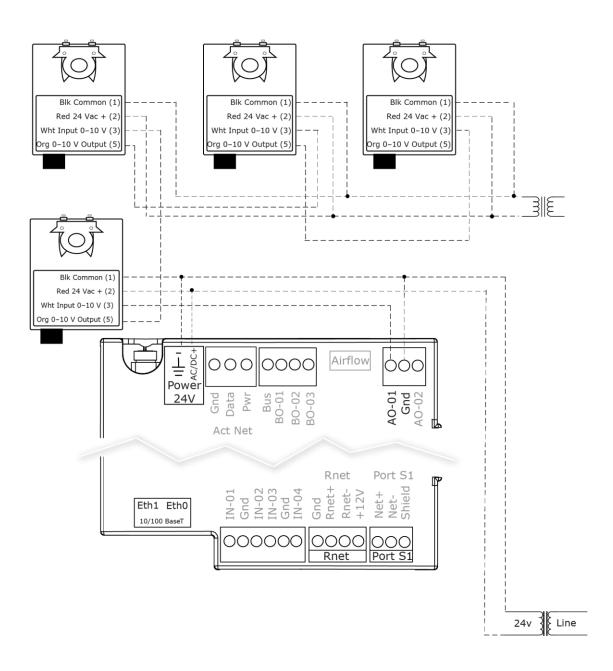
**NOTE** Maintain polarity if using the same power supply for more than one actuator.
