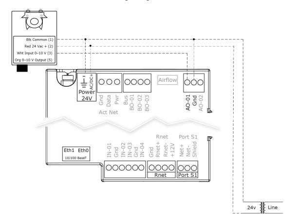
**NOTE** For proper operation and to prevent damage to the devices, use the same polarity for the actuator's power and the TV-VVTBP-E2's power.
