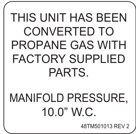
Fig. 7 — Propane Conversion Label – Propane Only
