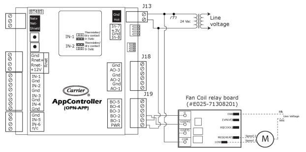
NOTE Configure Fan (G) Output Type as Fan On.
