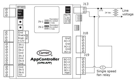
**NOTE** Configure Fan (G) Output Type as Fan Low.
