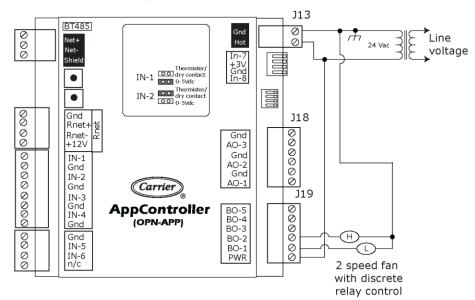
NOTE Configure Fan (G) Output Type as Fan Low.
