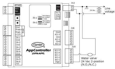
NOTE 2-position isolation valve is only available if Auxiliary Heat Type is None or Modulating.
