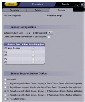
**Edit Increment** – Amount of offset in degrees for each press of the up or down arrows on the ZS or wireless sensor for setpoint adjustment.
