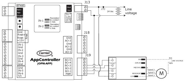
NOTE Configure Fan (G) Output Type = Fan On.
