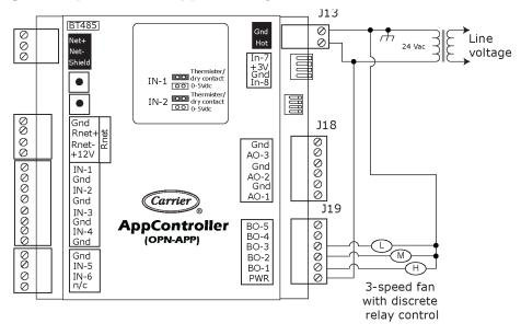
NOTE Configure Fan (G) Output Type = Fan Low
