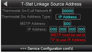
IP address, the MSTP address must be set to "0")
