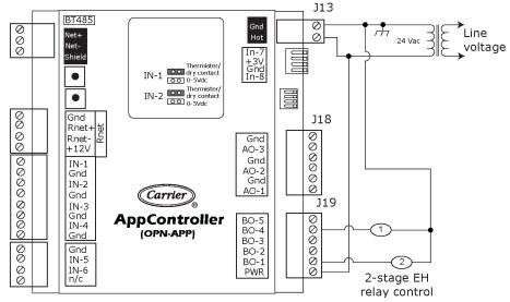
NOTE Only two fan speed are available when 2 EH stages are used. Configure # of Fan Speeds = One or Two.
