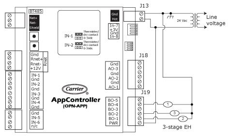
**NOTE** Only a single fan speed (on/off) is available when 3 EH stages are used. Configure **# of Fan Speed = One**. Refer to Motor Wiring for single speed field-supplied relay for wiring details.
