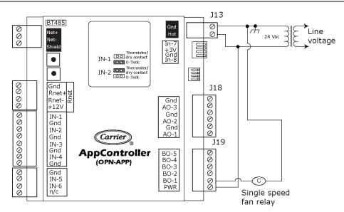
NOTE Configure Fan (G) Output Type = Fan Low
