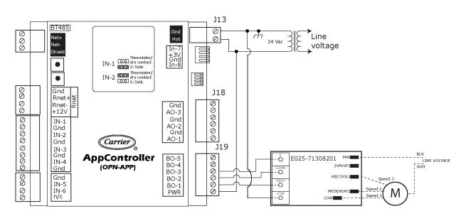
NOTE Configure Fan (G) Output Type = Fan On
