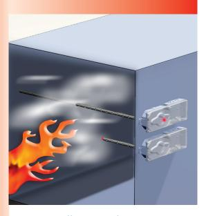
Don't Allow Smoke to Bypass The Sample Tubes!
