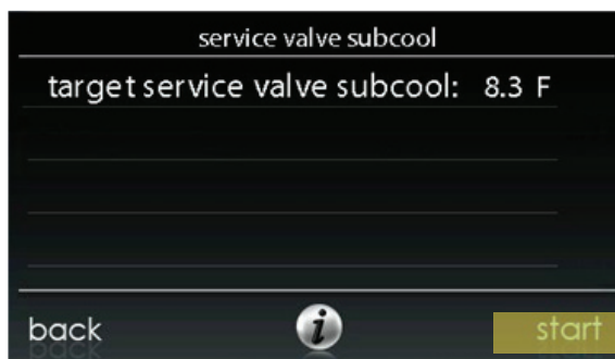
Fig. 16 - Service Valve Subcool Target Value
