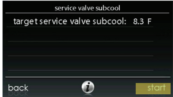
Fig. 16 - Service Valve Subcool Target Value
