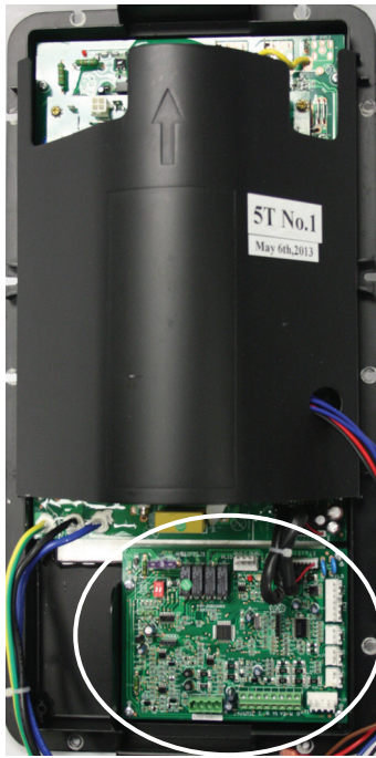
Fig. 23 - AOC (Application Operational Control) Board
