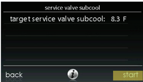
Fig. 10 – Service Valve Subcool Target Value A14574
