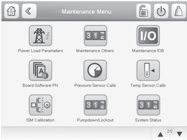
Fig. 35 — Maintenance Menu Calibration
