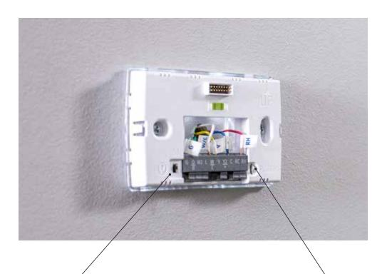
Nightlight switch Switching this "On" illuminates the thermostat base. Make sure you switch this to "Off" after installation so you can still operate this feature from the thermostat display.
