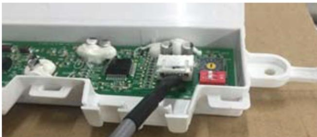
**Fig. 23 – Adaptor Board to Display Board Connection**
