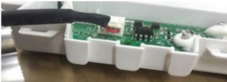
**Fig. 24 – Wired Controller port**
