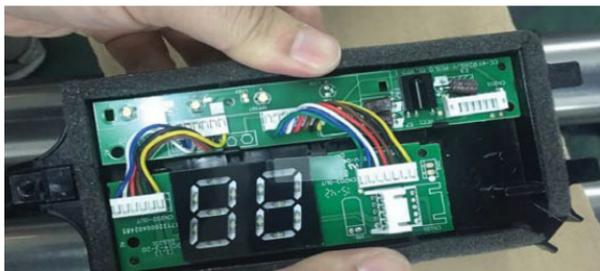
**Fig. 21 – Display Board Installed on the Display Board Holder**
