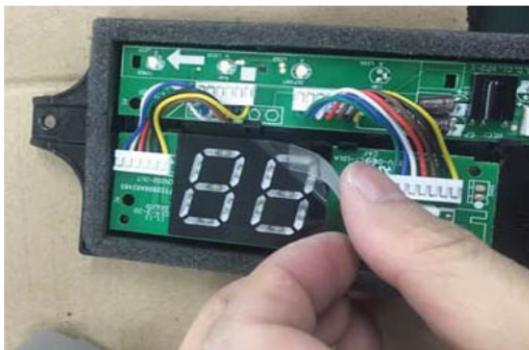
**Fig. 22 – Display Board Screen Cover**
