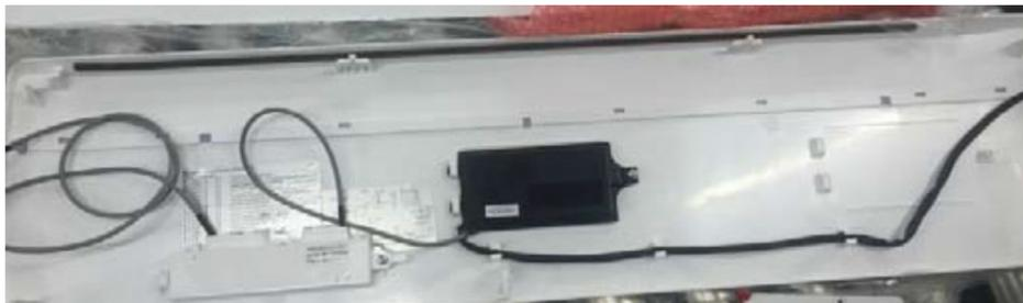
**Fig. 26 – Front Panel with New Display Board and Adapter Board**
