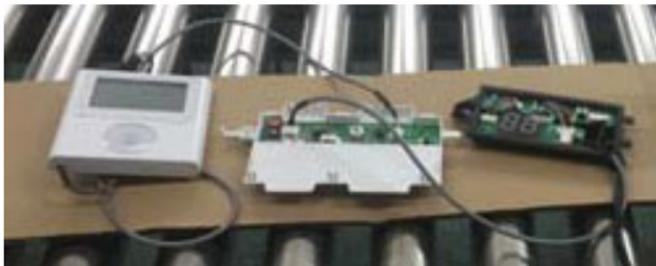
**Fig. 16 – Wired Controller, Adapter Board, and Display Board**
