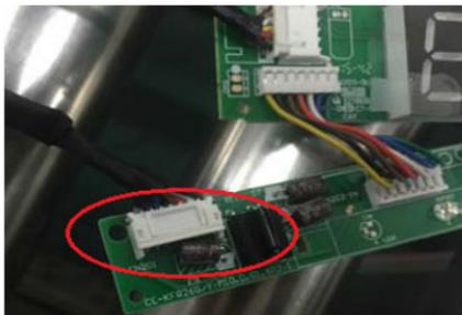
**Fig. 17 – CN201 Connection to the Main Control Board**
