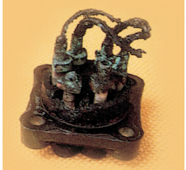
Photo showing acid attack on the compressor's terminal wires
