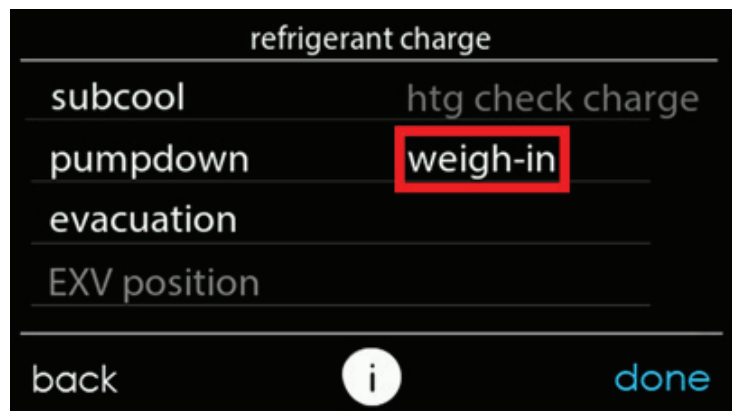
Fig. 15 – Weigh-in Option for charging below 65°F OAT and above 105°F OAT
