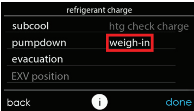
Fig. 15 – Weigh-in Option for charging below 65°F OAT and above 105°F OAT
