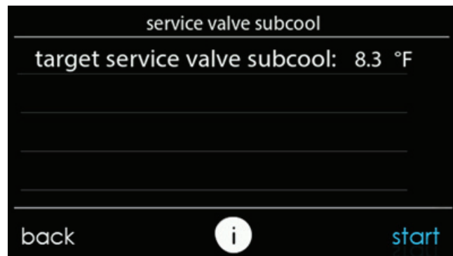
Fig. 13 – Liquid Service Valve Subcooling Target
