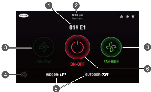
Fig. 15 — ERV User Interface of 40VM900005 Wired Controller
