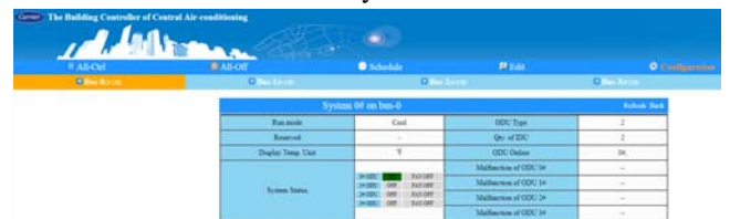
Fig. 25 —Additional Information on Refrigerant System
