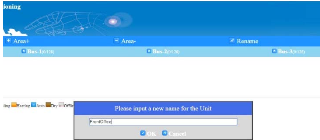
Fig. 19 —Tagging Units with Bus Number and Address
