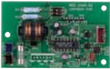
Size: 3.3 × 2.0 (in.) Install optional P.C. board in E-parts of the indoor unit.
