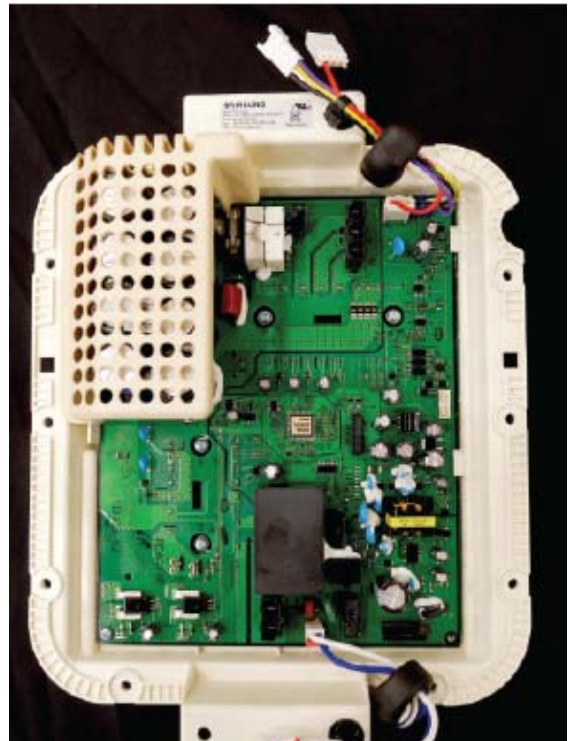
Fig. 21 – 4/5T VFD 5T VFD shown (4T VFD similar but not exact)
