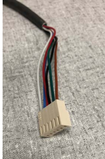
Fig. 31 – VFD to PCM Comm Cable (used on all models)
