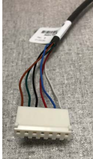
Fig. 31 – VFD to PCM Comm Cable (used on all models)
