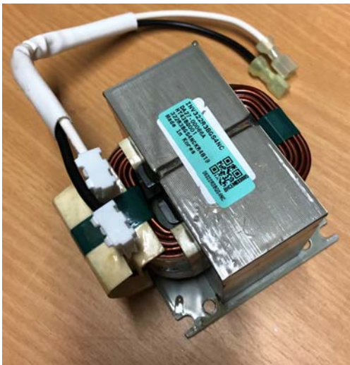
Fig. 27 – 2/3/4T Reactor (Note: 4Tuses 2 reactors)
