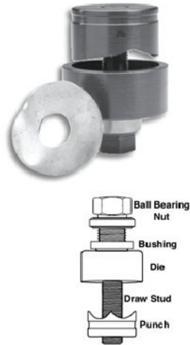
Fig. 1 - Greenlee® Knockout Punch
