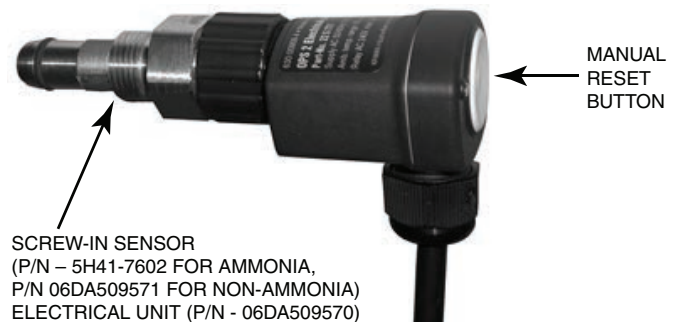
Fig. 13 — Oil Pressure Safety Switch Manual Reset Button
