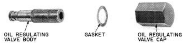
Fig. 33 — Oil Pressure Regulating Valve (Nonadjustable)
